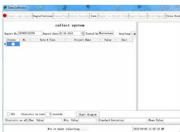
8. Press Continue Button- press button on SU 130 (e.g. FAST/SLOW) – Data acquisition Real Time starts
